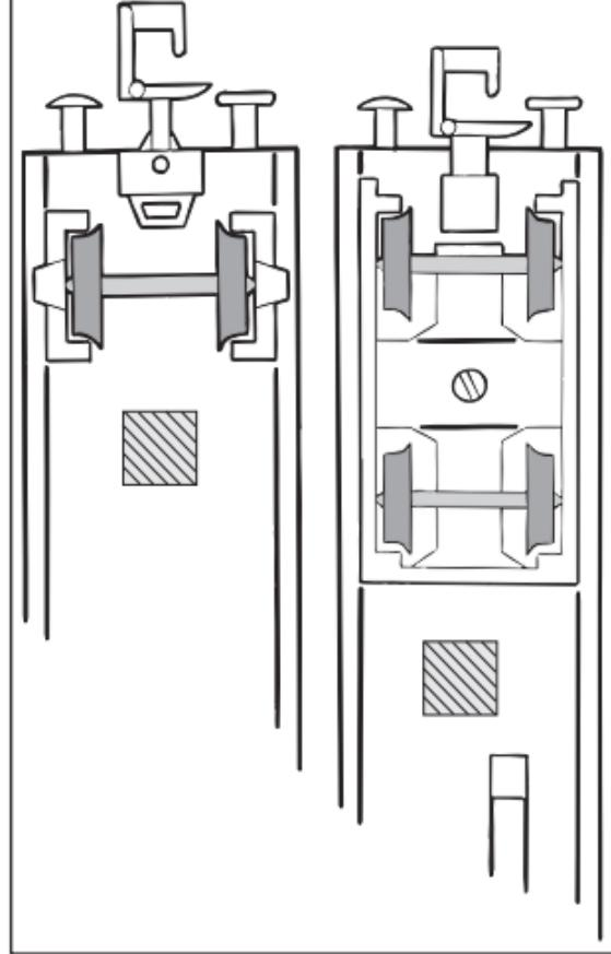
In order to ensure a troublefree switching function, the magnet is best positioned under the wagon chassis, near to an axle, or similary one of the bogies.
